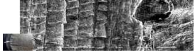
Figure 13. Machining traces of rough surface of axis and sub-layer fatigue glow
